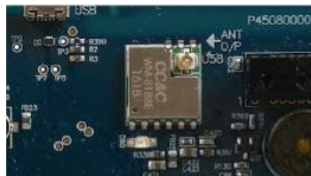
Figure 23 – Wi-Fi Integrated Circuit Antenna Connector
